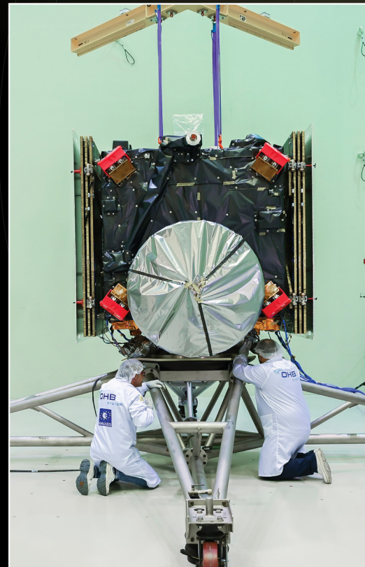
Acoustic testing – Hera was shut inside ESA's Large European Acoustic Facility, LEAF, to be blasted with noise. This is Europe's largest and most powerful sound system, fitted with a quartet of noise horns that can generate more than 154 decibels of extreme volume, to ensure Hera can survive the sound of its own launch.
