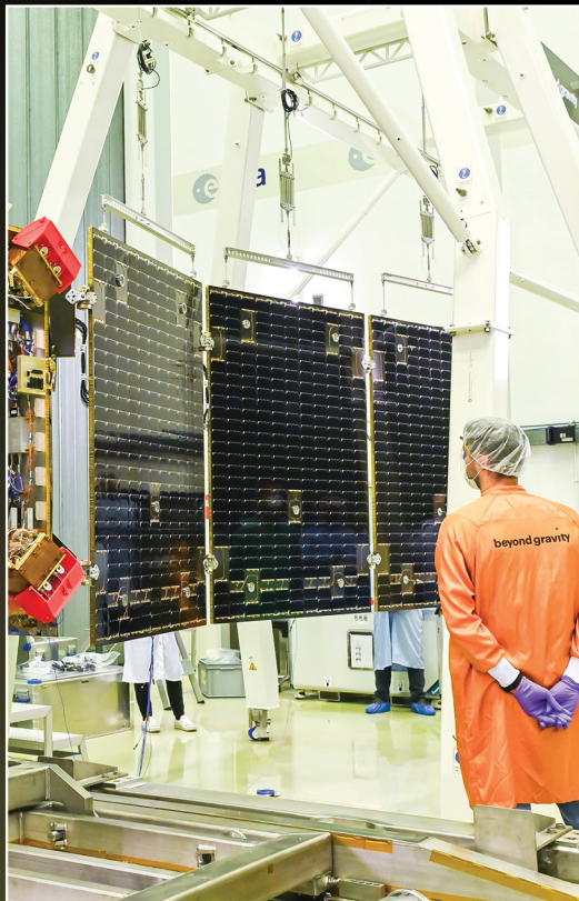
Solar array deployment – An initial 'cold deployment' saw the arrays unfolded by hand to confirm they fit correctly, followed by a 'hot deployment' where the arrays were deployed autonomously. The arrays were supported by a frame for testing because they are built for weightlessness.
