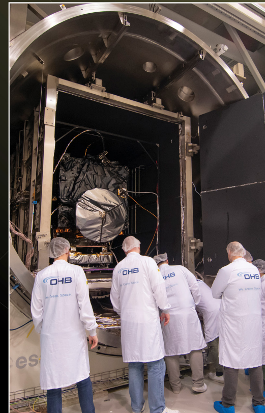
Thermal vacuum testing – Hera was placed in the Phenix vacuum chamber for test operations in space-grade vacuum, just a billionth of the atmospheric pressure outside. The spacecraft sat within a thermal tent inside the chamber so its surrounding temperature could be brought up and down, checking that Hera can maintain an optimal operating temperature.
